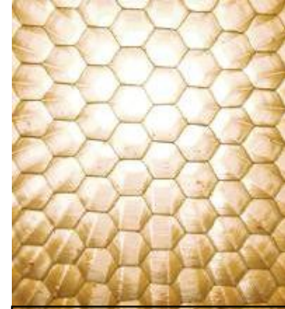
Photo 13 - Honeycomb sandwich panels (Source: Muehlenberg)
